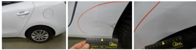
Rear bulkhead lining, Scratch(es), Smart repair
