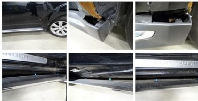
Sill outer R, Damaged, Le - Replace and paint
