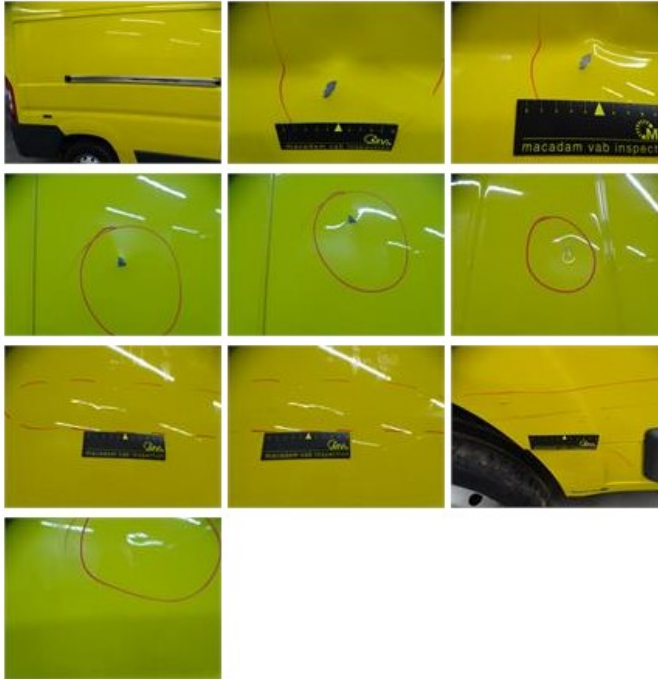
Trunk door panel L, Broken, E - Replace
