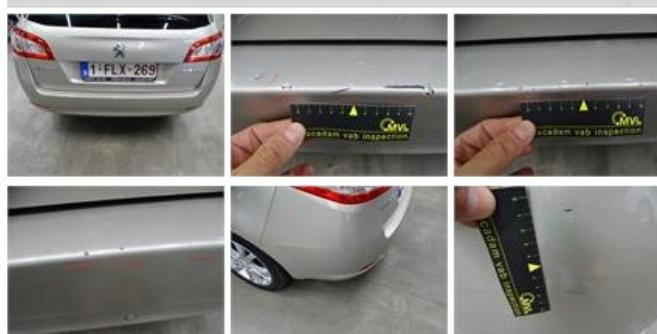
Rear spoiler, Chemical polution, LI - Repair and paint (complete)
