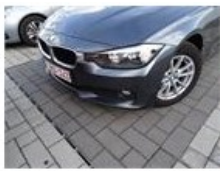
Wing R L, Dent(s), PDR - Knock out without painting 63,00
