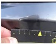
Wing R L, Dent(s), PDR - Knock out without painting 63,00
