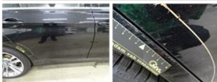
Rocker panel inner R R, Scratch(es), Acceptable 0,00
