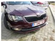
Bumper F, Hole, Le - Replace and paint
