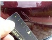
Bumper F, Hole, Le - Replace and paint
