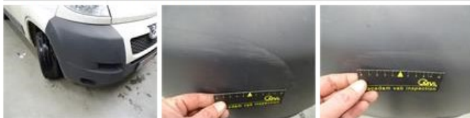
Sidewall RR (LCV), Scratch(es), It - Spot repair
