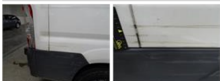
Roof pillar R, Dent(s), Le - Replace and paint
