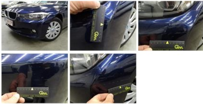
Bonnet, Scratch(es), LI - Repair and paint (complete)
