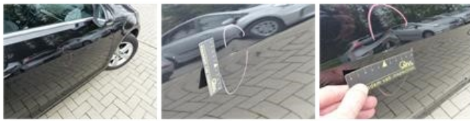
Wing F L, Hail damage, PDR - Hail
