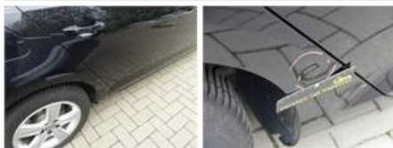
Wing R R, Dent(s), PDR - Paintless dent repair
