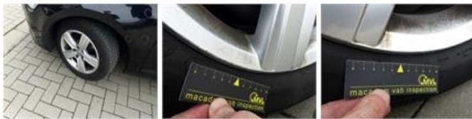
Wing R R, Dent(s), PDR - Paintless dent repair
