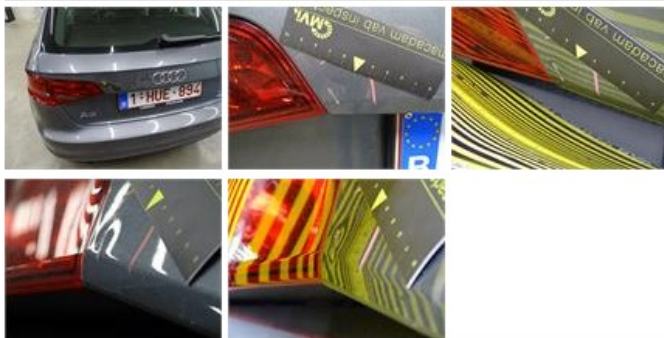
Wing F R, Dent(s), PDR - Paintless dent repair
