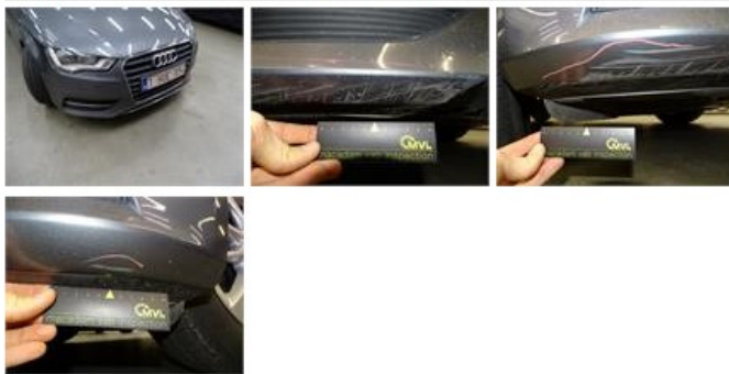
Trunk lid covering R, Scratch(es), Smart repair
