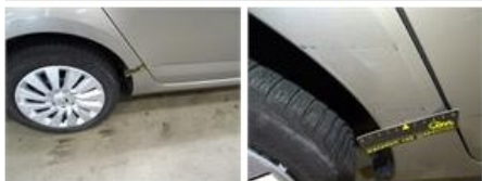
Wing F L, Dent(s) and scratch(es), LI - Repair and paint (complete)
