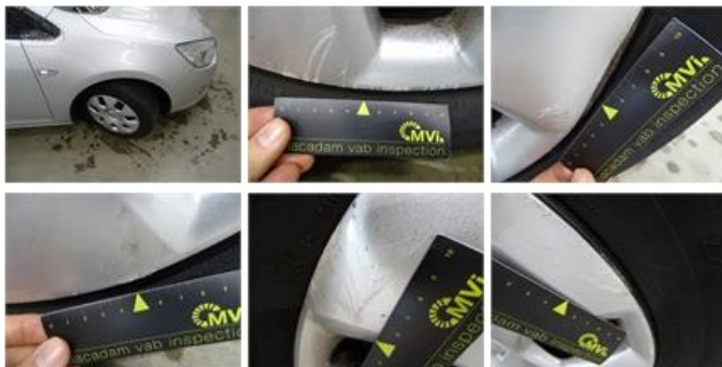
Wheel cover R R, Broken, E - Replace
