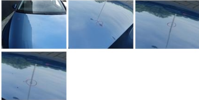
Tailgate, Hail damage, PDR - Hail
