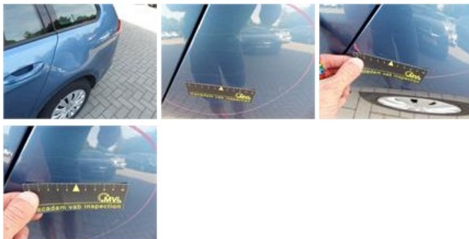
Roof pillar R, Hail damage, PDR - Hail
