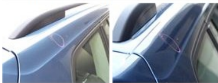
Roof, Hail damage, PDR - Hail
