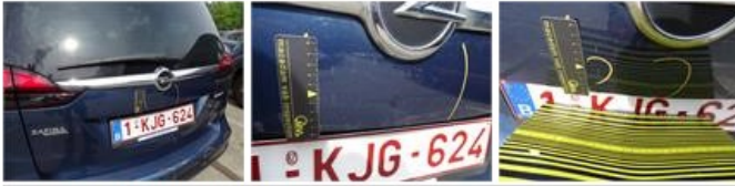
Wing R L, Dent(s), PDR - Paintless dent repair
