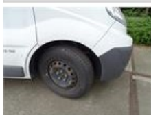
Wheel cover F L, Missing, E - Replace
