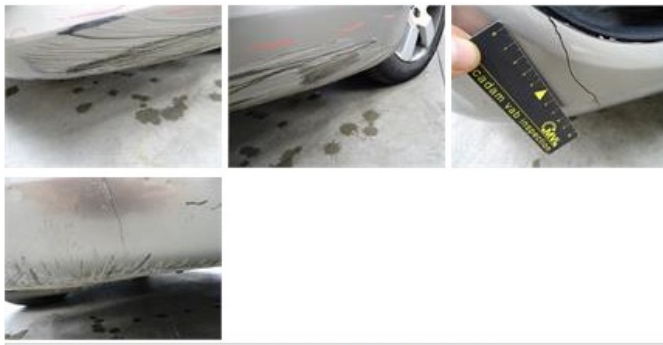
Rocker panel inner R R, Dent(s), LI - Repair and paint (complete)
