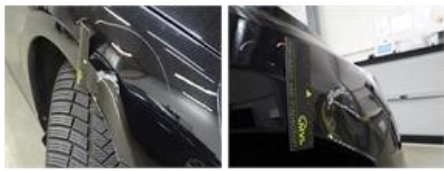
Floor covering F R, Hole, Smart repair
