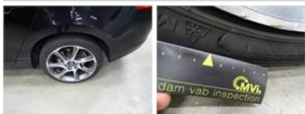
Tyre F L, Tear, E - Replace
