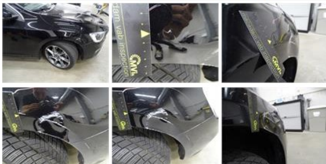
Wing F R, Dent(s) and scratch(es), LI - Repair and paint (complete)
