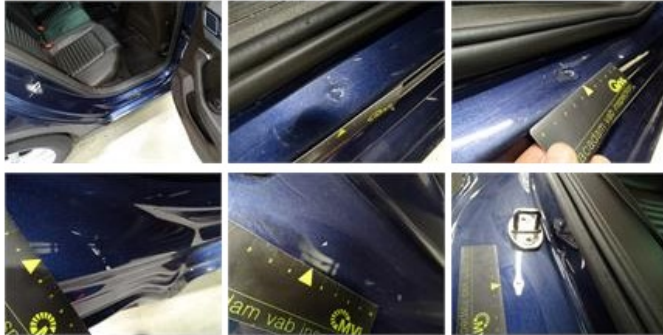
Door R R, Dent(s) and scratch(es), Acceptable
