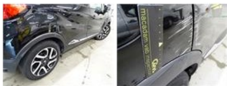
Bumper R, Crack, E - Replace
