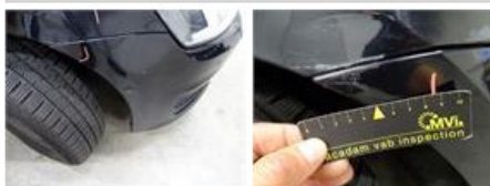
Reflector, Broken, E - Replace
