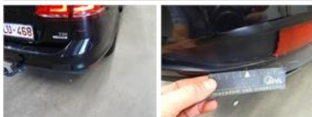
Rocker panel inner F L, Scratch(es), Acceptable
