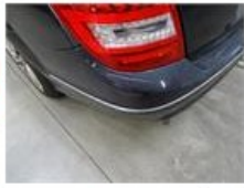
Bumper R, Dent(s) and scratch(es), Le - Replace and paint
