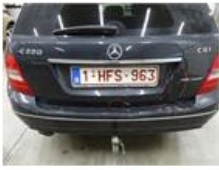
Bumper R, Dent(s) and scratch(es), Le - Replace and paint
