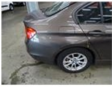
Wing R R, Dent(s) and scratch(es), LI - Repair and paint (complete)
