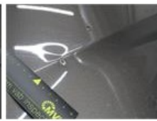
Wing R R, Dent(s) and scratch(es), LI - Repair and paint (complete)
