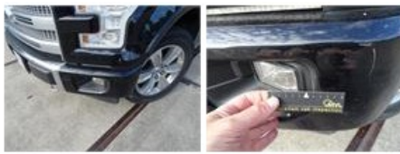
Bumper R, Crack, E - Replace
