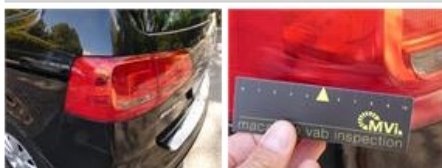
Foglight R, Broken, E - Replace
