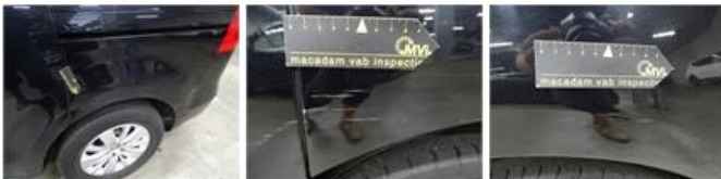
Rear Panel Internal Lining, Scratch(es), E - Replace
