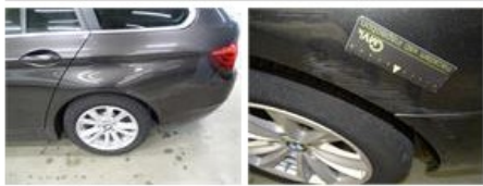
Door panel F L, Worn, Acceptable
