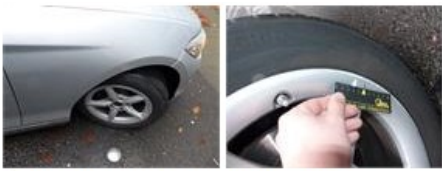
Wheel bolt cover R L, Missing, E - Replace
