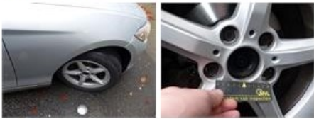
Wheel bolt cover F L, Missing, E - Replace
