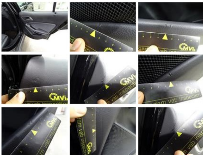
Door panel R R, Tear, Smart repair
