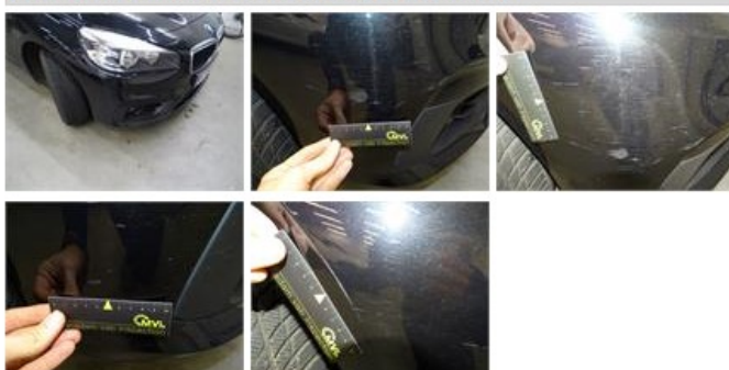
Bumper, Chemical polution, LI - Repair and paint (complete)
