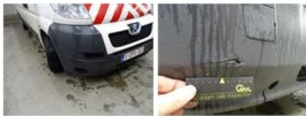
Grill frame, Broken, E - Replace
