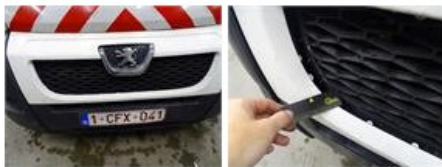
Engine protective plate, Broken, E - Replace
