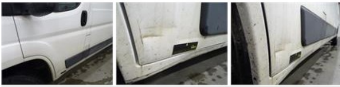
Separation wall, Dent(s), Acceptable
