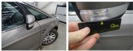
Door R L, Bad repair, Acceptable
