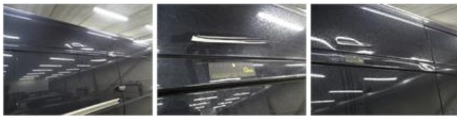
Mirror side blinker L, Broken, E - Replace
