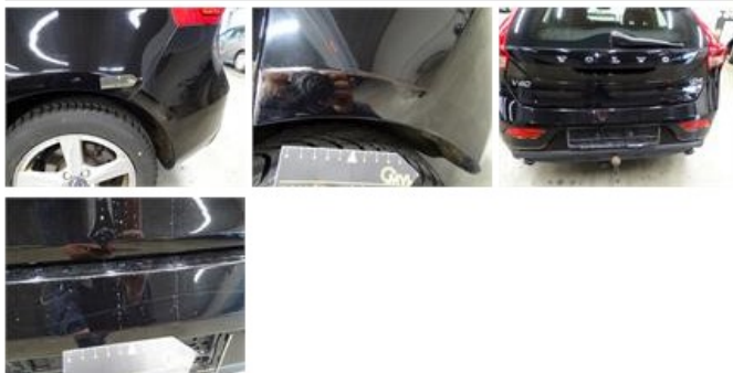
Bumper grille, Broken, E - Replace
